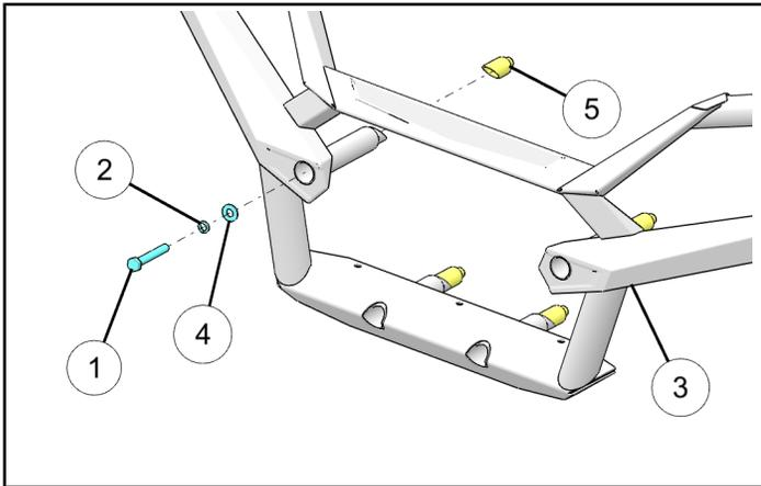
3. Install bumper assembly ③ onto front fascia (A) by inserting four wedge mounts into the holes in fascia. Push on bumper and tighten all four screws ①.
