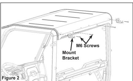
4. Install the three M6 bolts (PN 7518656) to secure the front of roof to upper frame on the vehicle. This will also help to compress the front seal (PN 5814086) for best sealing in inclement weather. Torque to 16 ft-lbs. (21.7 Nm). Figure 3.
