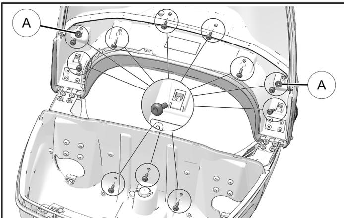
4. Install nine screws ③ to secure pads to trunk. Install two screws ③ with reserved washers ① and cable eyes. Torque to specification.
