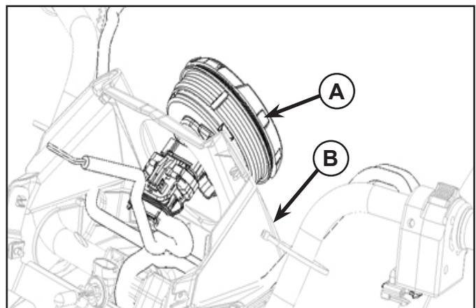
3. Align audio mount bracket (5) on the pod (B) and use as template to drill the holes (E) of dia 5/16" as shown in figure.
