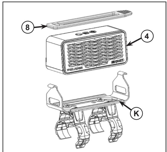
3. Snap fit bluetooth speaker assembly on to the ROPS tube (1.75" Dia) at any required location.
