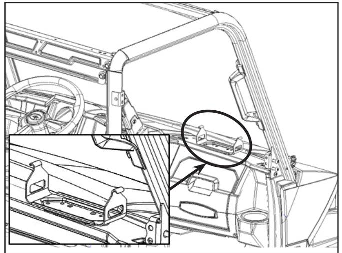
2. Before installing audio mount base (6), place and align the pad (9) with holes on dashboard and audio mount as shown in figure.
