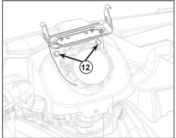
7. Use rubbing alcohol, pledge or other temporary lubricant on the rubber gasket, both sides. Push back bezel and cluster assembly (F) to fix onto the upper pod as shown in figure.
