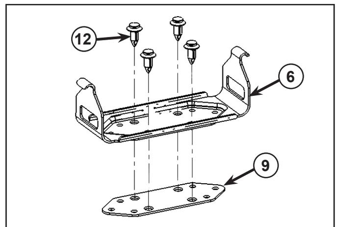
3. Mount audio mount base (6) with four tuflok rivets (12) on the dash panel as shown.
