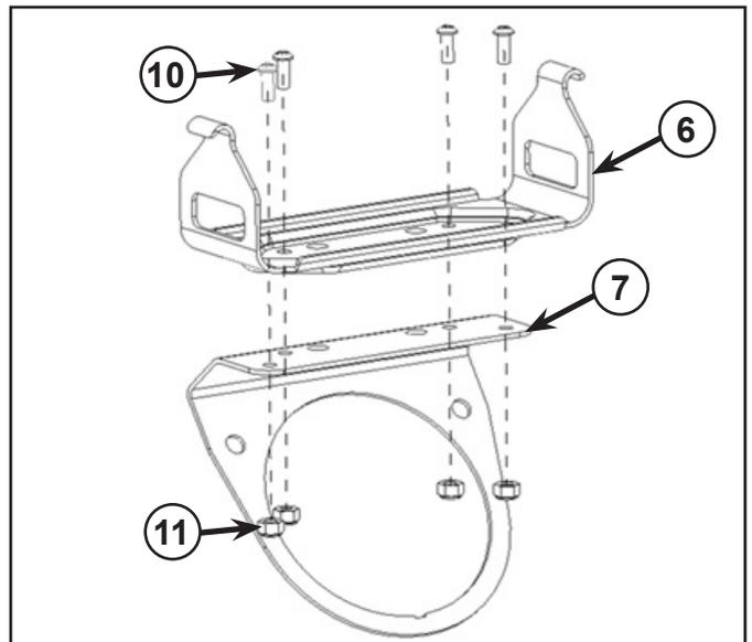
6. Align and Install audio mount bracket assembly on the pod using two tuflok rivets (12) as shown in figure.
