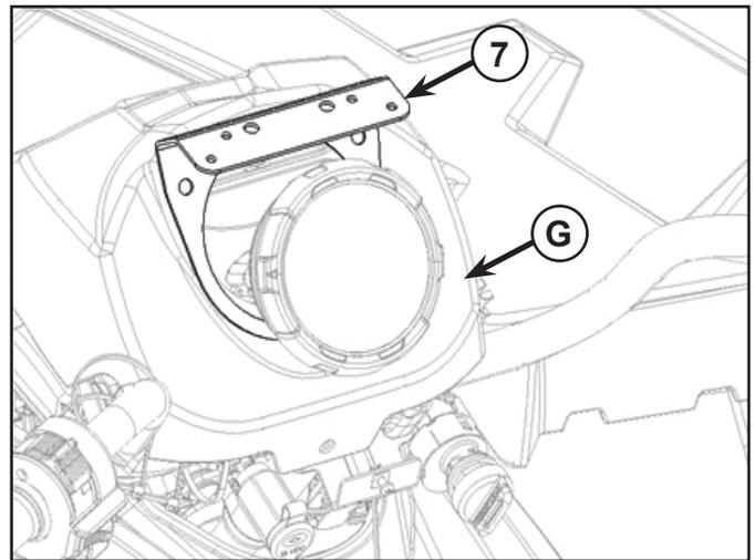
5. Fasten audio mount bracket (7) with audio mount base (6) using four screws (10) and nyloc nuts (11). Tighten screws until snug.
