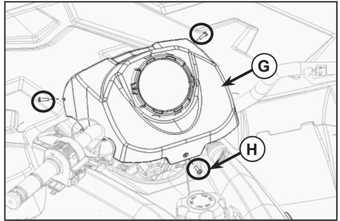
4. Align audio mount bracket (7) with pod (G) and use as template to drill the holes of dia 5/16" as shown in figure.
