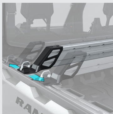
3 SLIDE TO DESIRED LOCATION
