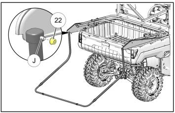
d. Install nut <sup>(2)</sup> to each stud <sup>(1)</sup>, but do not overtighten. Pole assembly must be free to rotate on studs.
