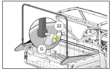
d. Install nut <sup>(2)</sup> to each stud <sup>(6)</sup>, but do not overtighten. Pole assembly must be free to rotate on studs.
