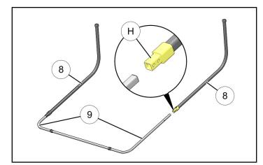
c. Loosely install one side of pole assembly to stud ① on bracket, then install opposite side.
