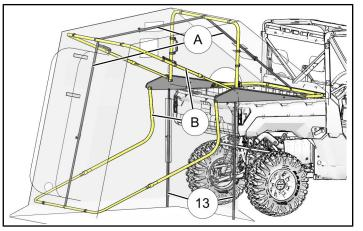
3. Depress lock buttons (LH and RH sides) on Ushaped DOOR and BOTTOM pole assemblies (B), then fully collapse pole frames.
