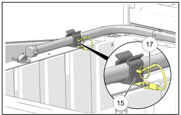
b. Detach end hook (A) from MIDDLE STRAIGHT SECTION pole (3).
