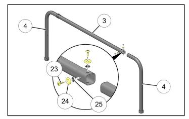
b. With pole assembly in upright orientation, loosely install one side of pole assembly to stud
