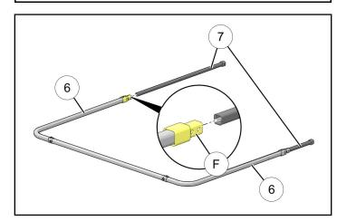
With pole assembly in upright orientation, loosely install one side of pole assembly to stud <sup>©</sup> on bracket, then install opposite side.
