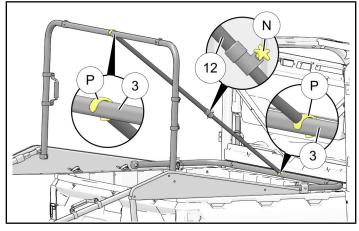
d. Extend U-shaped door pole assembly (1) rearward until lock button engages FIRST hole
