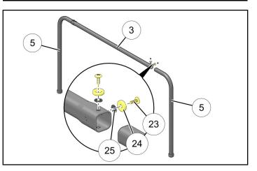
b. With pole assembly in upright orientation, loosely install one side of pole assembly to stud () on bracket, then install opposite side.
