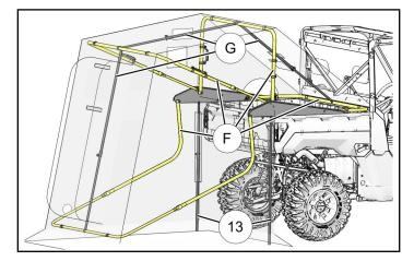
5. Secure shelter to U-shaped pole assemblies using hook and loop strips.
