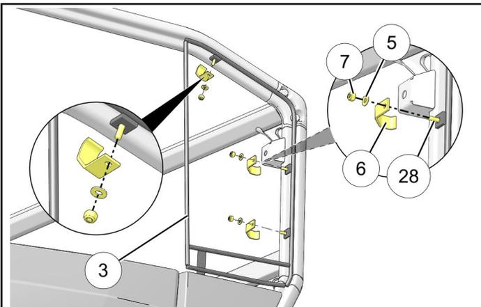
3. Loosely install bolster panel ③ post to vehicle frame using bolster panel bracket ⑧, screw ④, washer ⑤, and nut ⑦.
