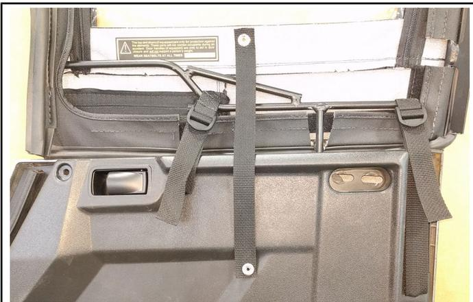
7. Install pull strap (27) to upper door (2) by wrapping each end of strap around door frame, then snapping into place as shown.
