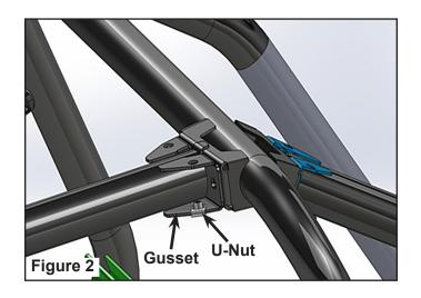
2. Install the mounting bracket using the top ROPS bolt at the bottom of the B-pillar. Figure 3.
