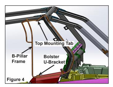
4. Attach the top mounting bracket loosely to the U-nut on the top B-pillar gusset using a Phillips head screw and a flat washer. Figure 5.
